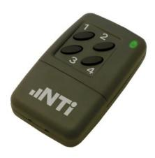
The XL2 Input Keypad offers four keys to trigger an event recording or categorize noise during measurements. It is an accessory to the XL2 Audio and Acoustic Analyzer.
